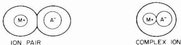
FIGURE 3.3. Diagram of an ion pair and a complex ion.
