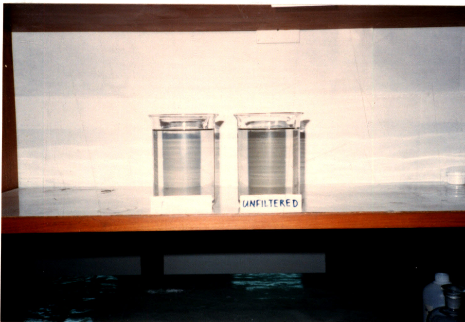
Fig P6 Filtered and unfiltered effluent samples of PAC unit
