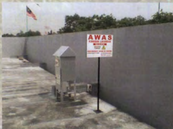
Plat 5.6 Johor : Stesen Pengawasan Manual Air Quality Monitoring (MAQM)
