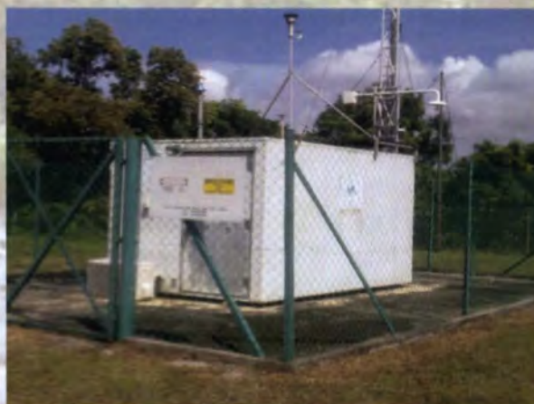
Plat 5.7 Johor : Stesen Pengawasan Continuous Air Quality Monitoring (CAQM)
