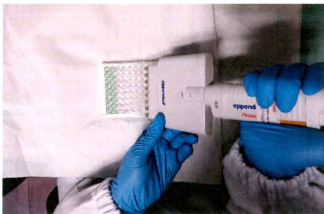
Figure 3.21: One of the steps in ELISA using a multichannel pipette
