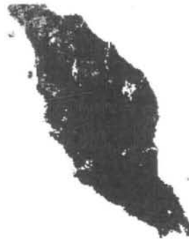
Figure 2.18: The final cloud mask for Malaysia for 30 January 2004. Cloud pixels are masked red; cloud-free and water body pixels are masked grey and white respectively.
