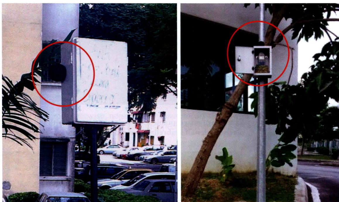
Figure B-15: Examples of unacceptable use of sound level meter installed in a casing as an alternative to permanent noise monitoring units
