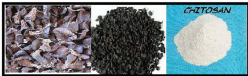
FIGURE 11.1 The figure demonstrates the pictorial view of palm oil shell, palm oil shell charcoal, and chitosan which is after all coated on the palm oil shell charcoal and can be used as adsorbent.
