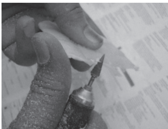
FIGURE 3.3 Sample grinding with the help of metallic bur attached to lab micro motor.
