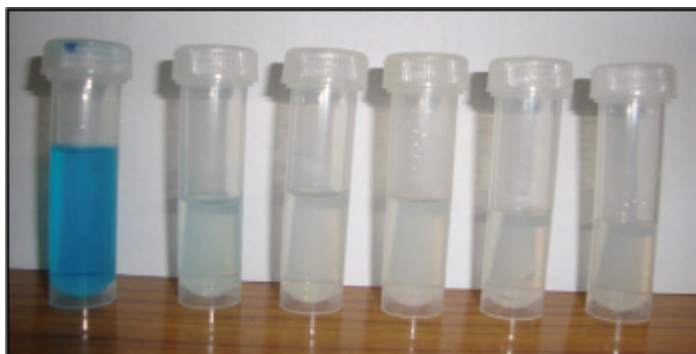
FIGURE 14.8 Dye (RB 21) removal in different time interval using \text{MnO}_2 -coated fly ash.
