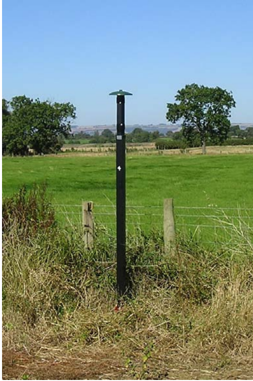
Figure 1: An example DustScan monitoring installation.
