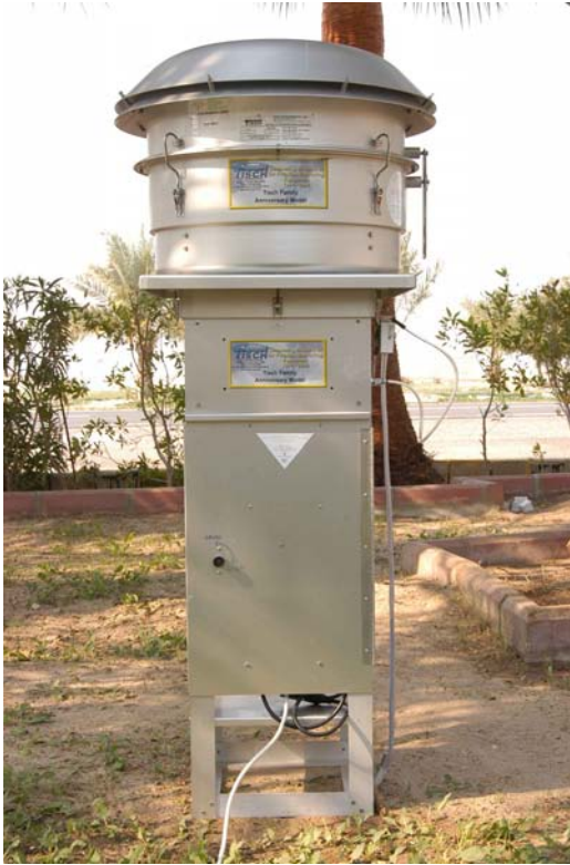
Figure 4: The PM10 high volume air sampler in use at A17.
