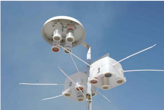
Figure 2: Triplicate set of the passive samplers.
