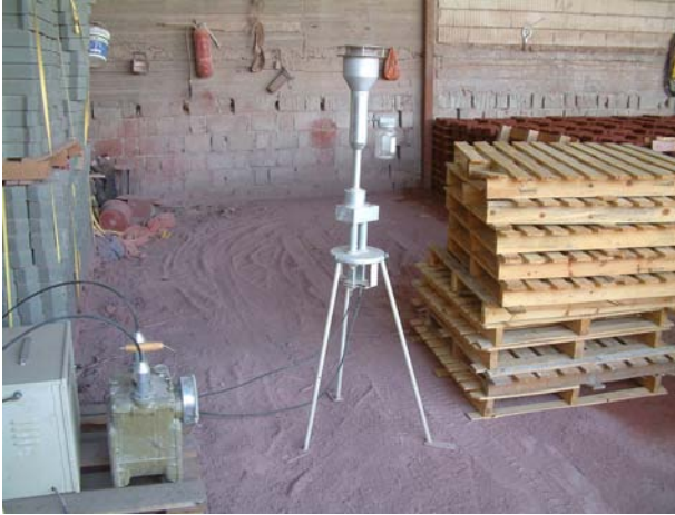
Figure 3: A Dichotomous sampler in a block workshop.
