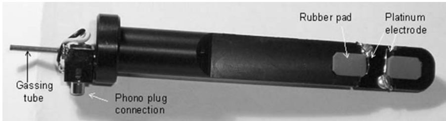
Fig. 1. Stimulators used for muscle stimulation. Body of device is made from Delrin plastic and is designed to fit into a Falcon 2059 (17 × 100) tube. Tube at top extends to bottom of device to allow gassing of media. Phono plug-type connector on top of device is attached to wires that run down the back of device and are attached to platinum wires with screws at right. Muscles are pinned to rubber pads at right and lie in between electrodes.
