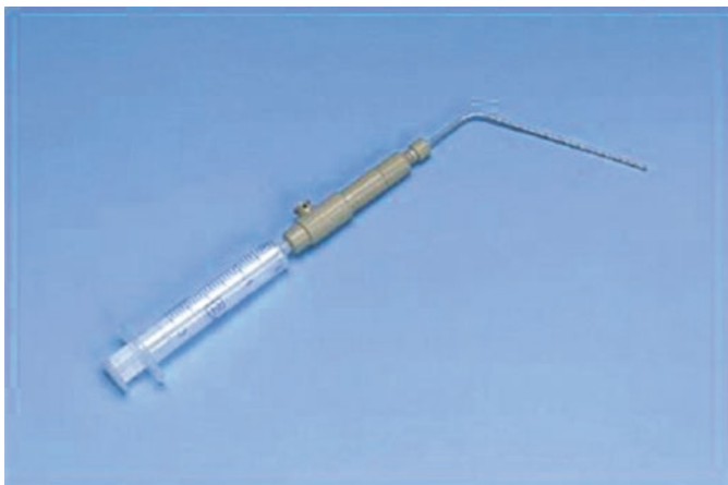
Fig. 2.14 Penn-Century Model DP-4 M dry powder insufflator with attached syringe
