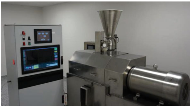
Fig. 13.3 Kinetisol® KC254C Compounder for semi-continuous operation (Courtesy of Dispersol Technologies)
