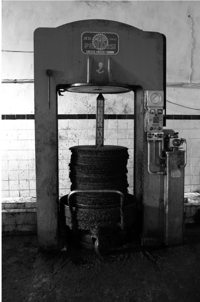
Figure 6.3 Olive press showing fibre discs (Wikipedia).
