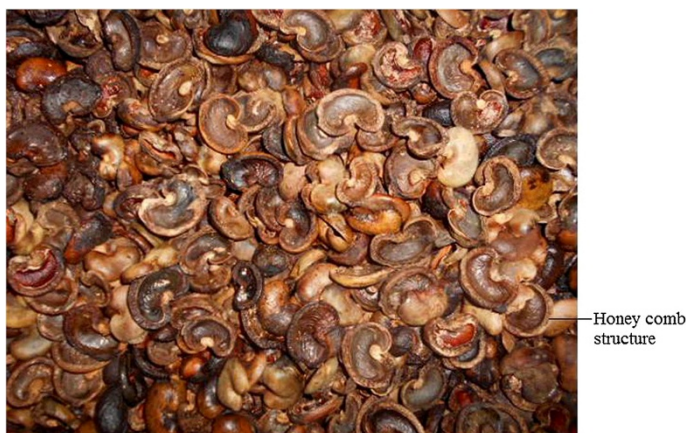
Fig. 2 Picture of cashew nut shells showing a honeycomb structure
