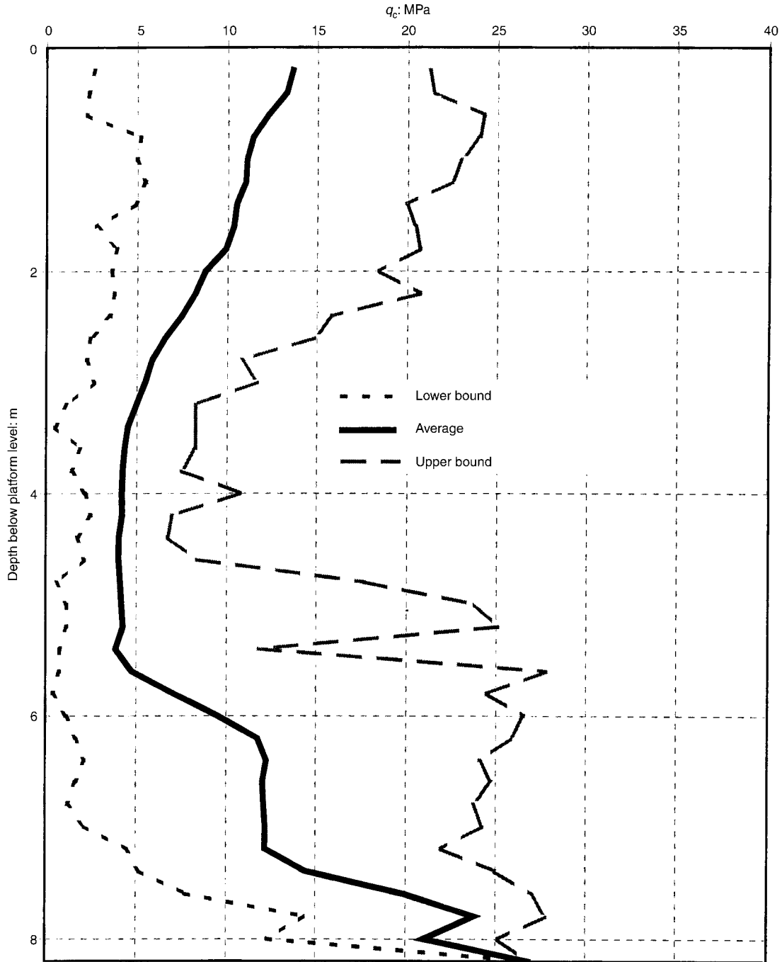
Fig. 10. Pre-treatment reclamation CPT tip resistance ( q_c profiles) (85 results)
