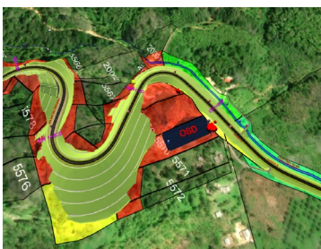
On Site Detention (OSD) and Final Discharge
