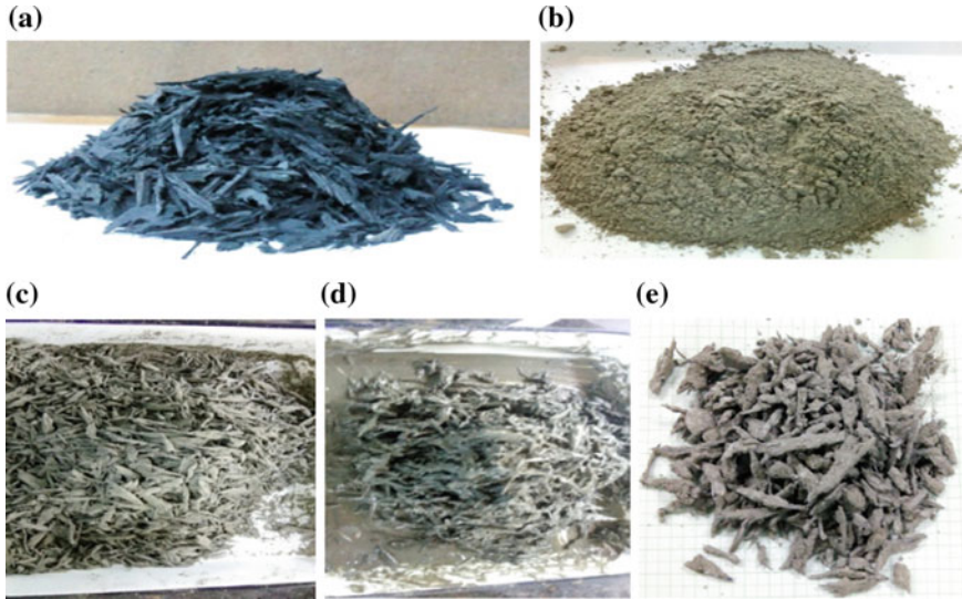
Fig. 3 Stages involved in the preparation of cement coated tyre fibres. a Tyre fibres, b Ordinary Portland Cement (OPC_53), c dry mixtures of tyre fibres and cement, d wet mixture of tyre fibres and cement, e cement coated tyre fibres
