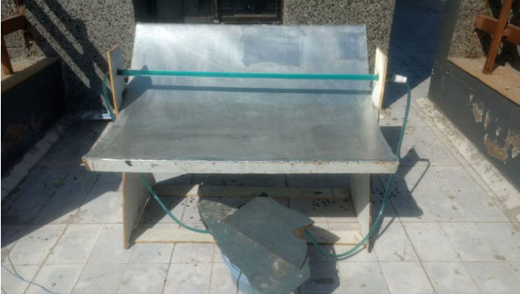
Fig. 1 Setup of parabolic trough collector
