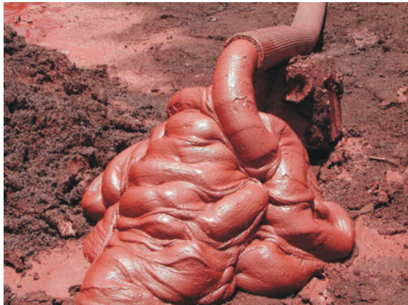
Fig. 5.7 Paste Tailings. Source Mark T. Biesinger/ WesTech Engineering, Inc., [17]
