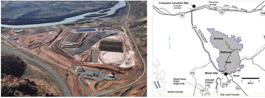
Fig. 5.9 left: uranium tailings pond Moab directly adjacent to the Colorado River; right: section of the transport plan. Source [26], public domain
