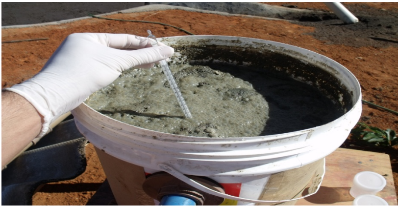
Figure 5. Temperature measurement of the effluent.
