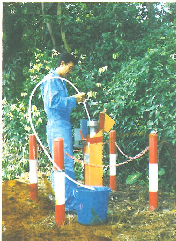
Photo 10: Groundwater sampling (DOE Photo Library)
