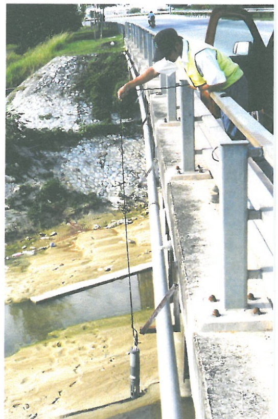
Photo 9 : River Water Quality Manual measurement (DOE Photo Library)
