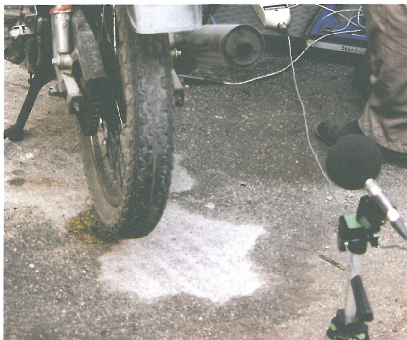
Photo 7 : Noise Level Monitoring (DOE Photo Library)
