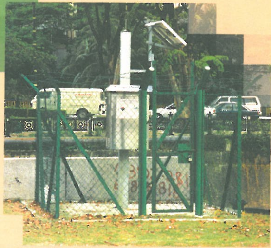
Photo 12 : Continuous River Water Quality Monitoring Station (DOE Photo Library)
