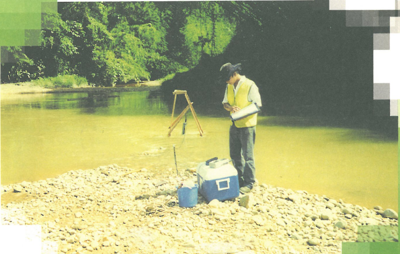
Photo 9 : River Water Quality Manual Measurement (DOE Photo Library)
