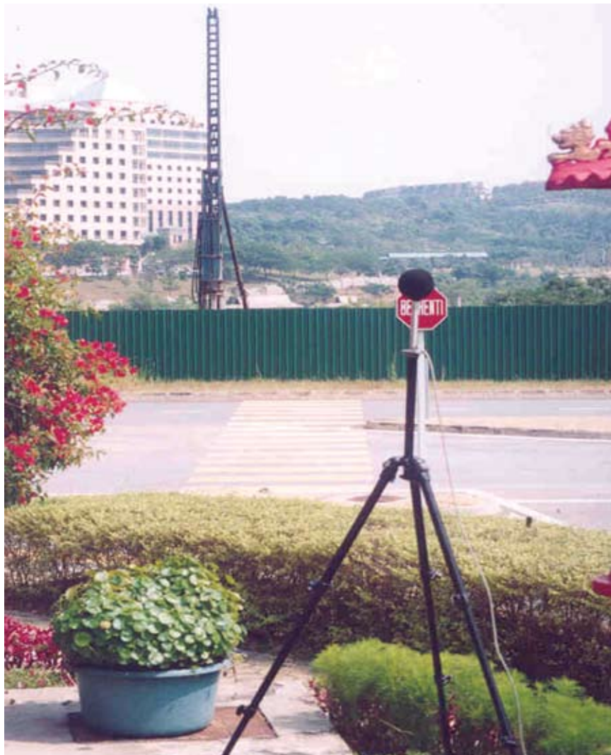
Noise monitoring – Construction site piling (DOE photo library)
