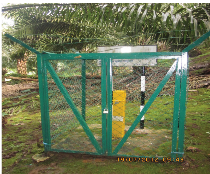
Stesen Pengawasan Kualiti Air Tanah di Yong's Farm, Tawau (guna tanah pertanian) Groundwater Monitoring Station at Yong's Farm, Tawau (for agriculture land use)
