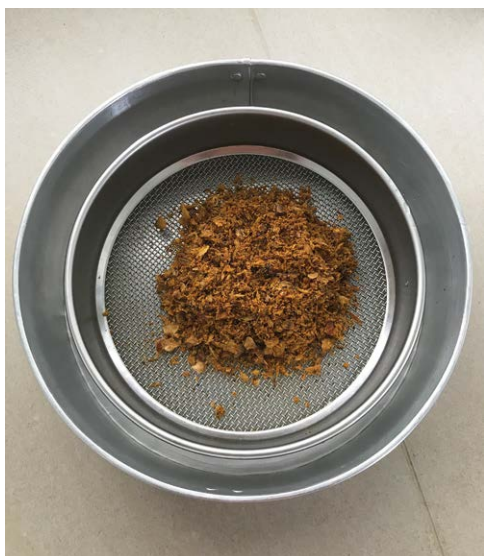
Fig. 7.4. Step 4: Place the ground dry mesocarp into a round aluminium sieve dish.
