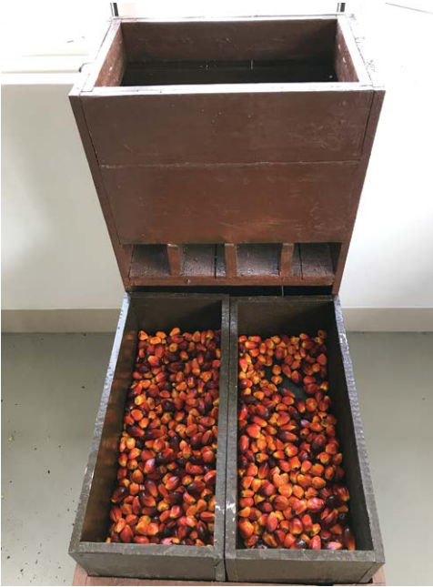
Fig. 5.2. Step 2: Open the floor of randomization box to allow fruit to fall into collecting boxes.
