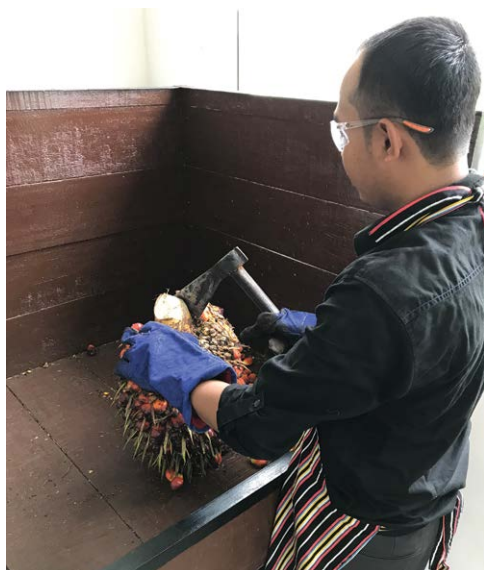
Fig. 4.4. Step 4: Chopping the bunch with an axe on a chopping table to separate and remove all the spikelets.
