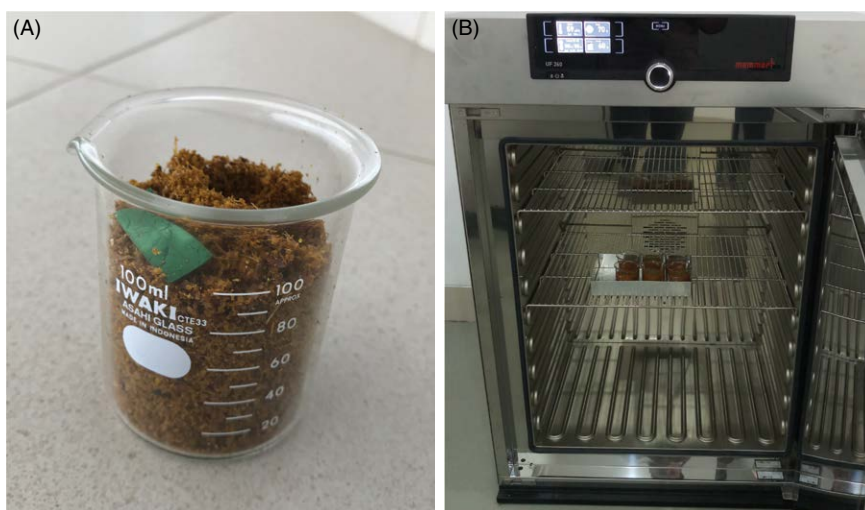
Fig. 7.6. Step 6: A) Store the ground dry mesocarp in a glass beaker; B) Dry the ground dry mesocarp in an oven.
