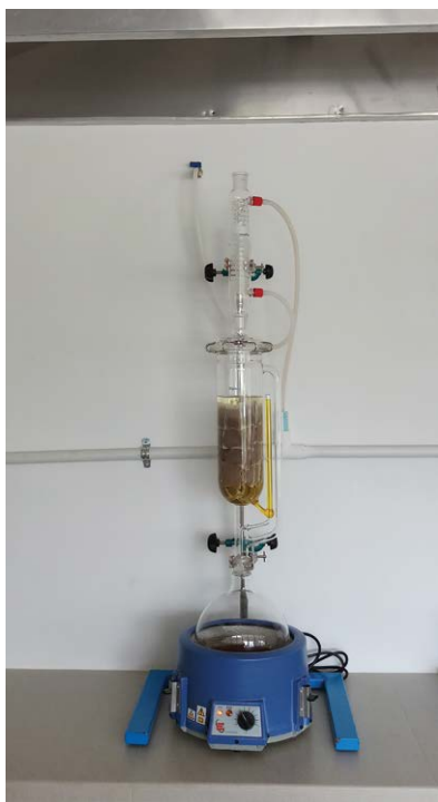
Fig. 7.10. Step 10: Extraction of enveloped dry mesocarp samples using a soxhlet extraction system.
