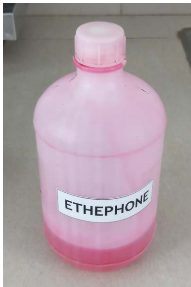
Fig. 4.17. Bunch physical analysis material: ethephon, used to ferment the bunch which helps in loosening and detaching spikelets and fruits.
