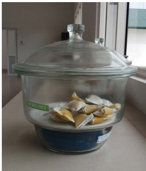
Fig. 7.9. Step 9: Keep the enveloped mesocarp samples in desiccator prior to oil extraction if not used immediately.
