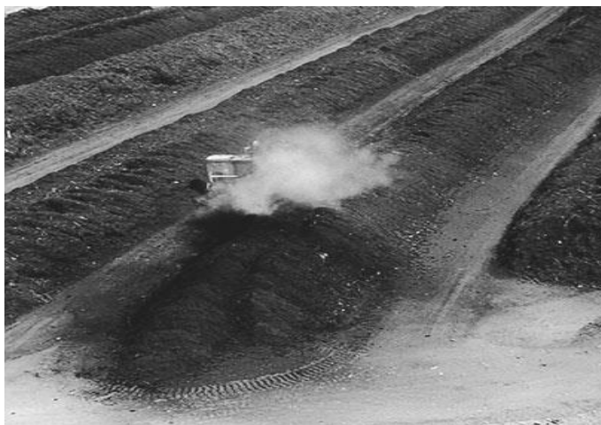
Figure 11. Windrow composting of MSW.
