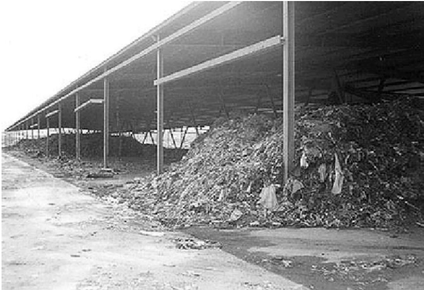
Figure 3. Un-sieved compost full of foreign materials such as plastics and metals.
