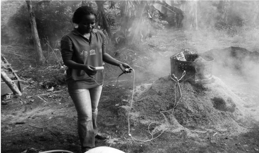
Figure 8. Monitoring of temperature in a biochar production in Ghana (local method).
