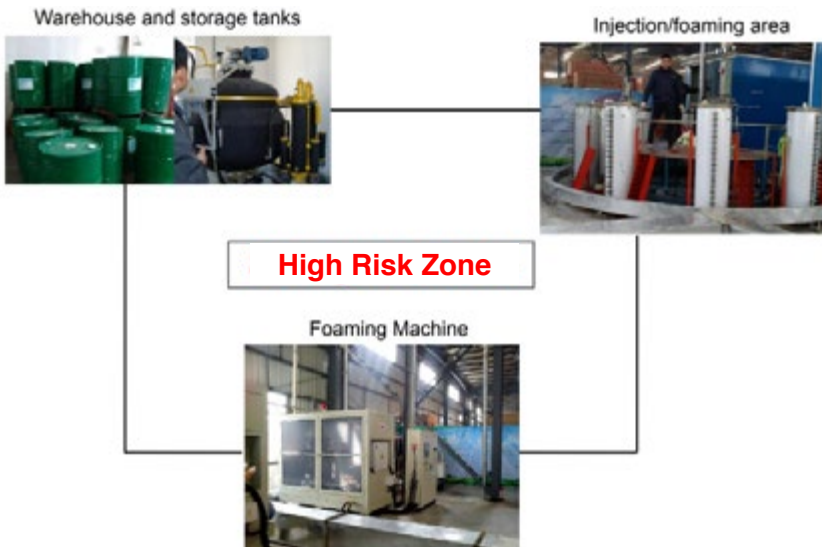
Figure 6.3: High Risk zones for pre blended cyclopentane system
