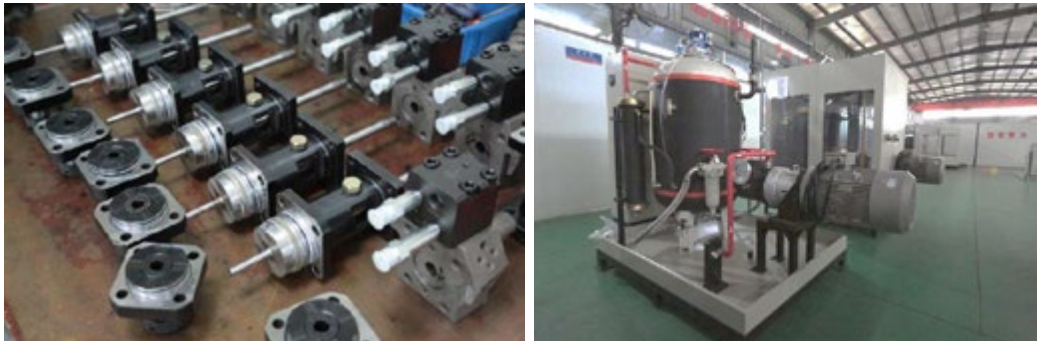
Figure 6.4: The mixing head and the fully automated injection machine for cyclopentane (C5) adoption.
