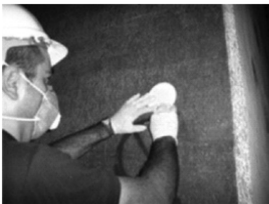
Figure 7.2 Sampling of contamination by the wipe test technique.
