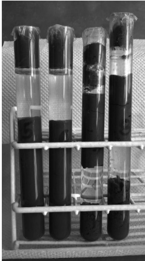
Figure 7.11 Behavior of selected MNPs (left) versus \text{AlSO}_4 flocculant (right).
