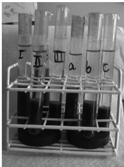
Figure 7.12 Demulsification after 6 months (magnetically assisted).
