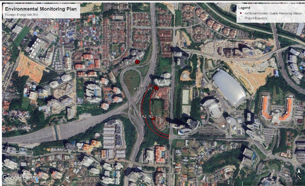
Figure 6.6: Baseline Monitoring Stations for Air Quality, Noise Level and Vibration Quality
