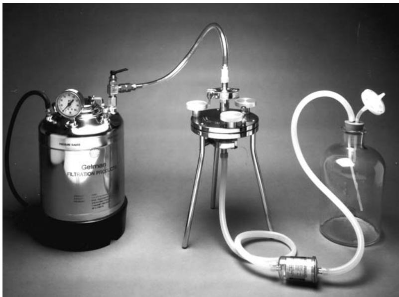
Figure 7.10 Sterile filtration of a small-volume pharmaceutical solution with a 142 mm plate-and-frame filter used as a prefilter in front of a small disposable cartridge final filter. From Gelman Science
