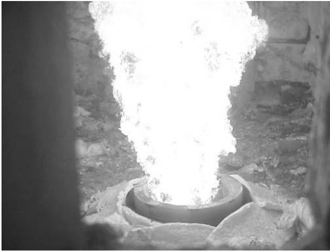
Figure 3.6 Example of a highly luminous heavy oil flame. (From Ref. 4. Courtesy of John Zink Co.)
