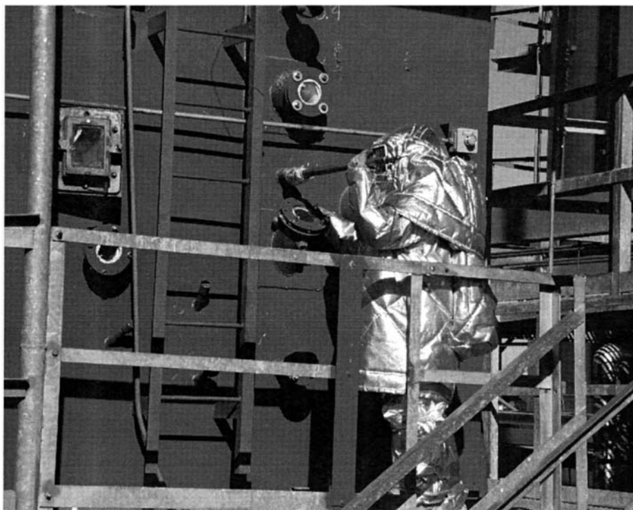
Figure 11.16 Protective clothing for high-heat environments.
