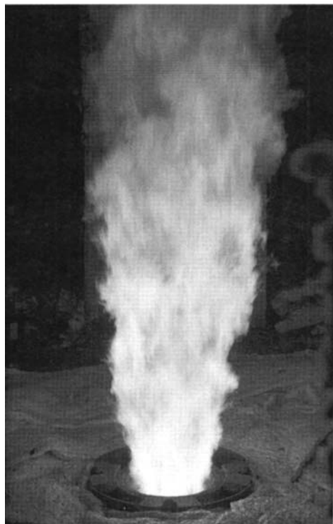
Figure 12.18 Burner firing heavy oil with new oil atomizer. (From Ref. 17. Courtesy of John Zink Co. LLC, Tulsa, OK.)
