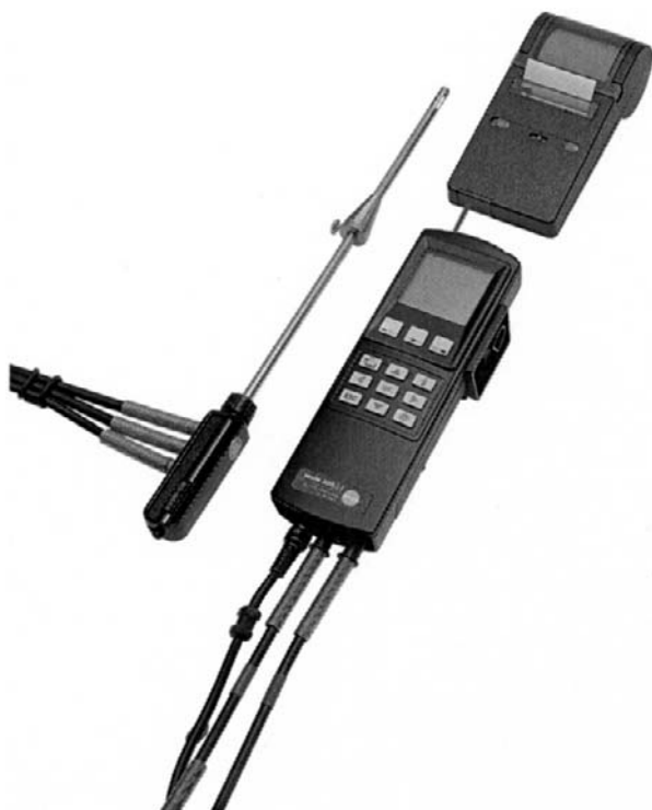
Figure 6.47 Portable gas analyzer. (Courtesy of Testo, Flanders, NJ).
