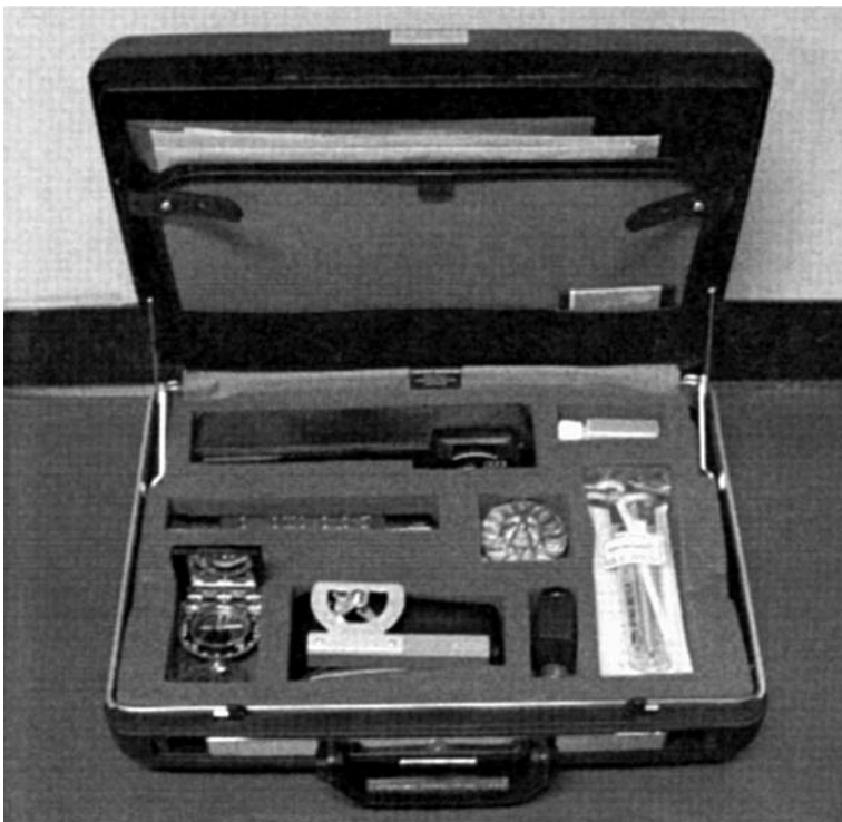
Figure 5.49 Field kit for making gas emission measurements. (Courtesy of ETA, Garner, NC.)
