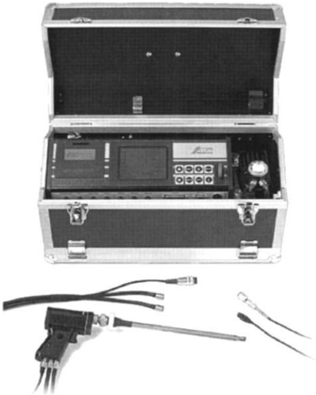
Figure 5.50 Portable gas analyzer. (Courtesy of ECOM, Gainesville, GA.)
