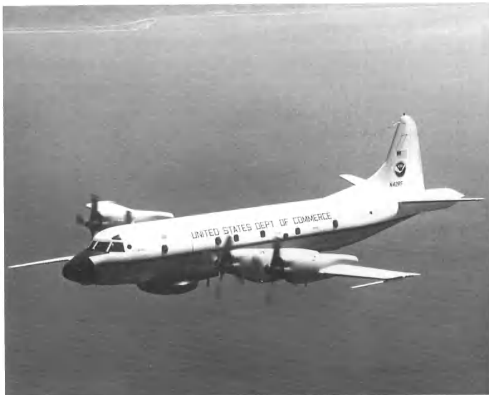
Fig 1. The National Oceanic and Atmospheric Administration WP-3D Orion research aircraft used in the Arctic Gas and Aerosol Sampling Program. This aircraft is capable of 10–12 hour research missions with a range of 3,000+ nautical miles.
