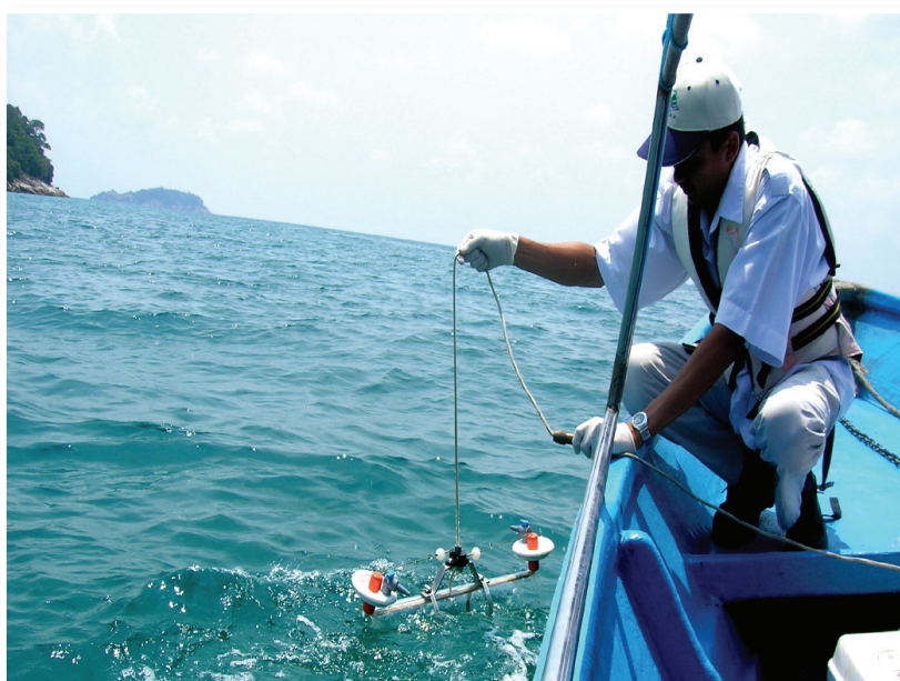
Persampelan Kualiti Air Marin Menggunakan Van Dorn Sampler Marine Water Quality Sampling By Using Van Dorn Sampler
