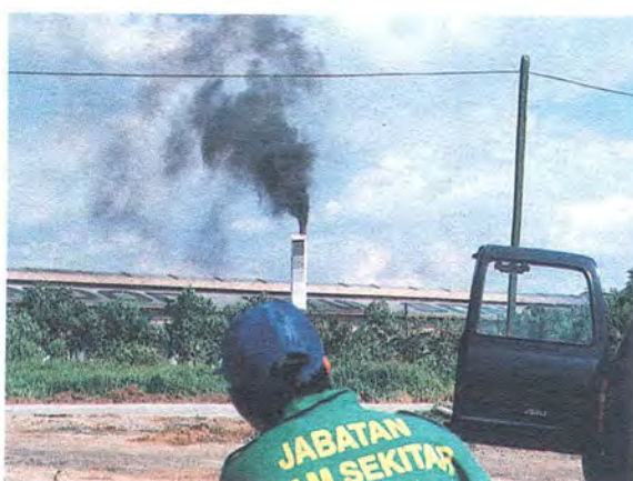
Visual observation of black smoke emission using Ringlemann Chart
