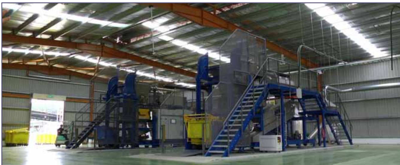
Figure 3: Microwave machine for sterilisation of clinical waste at Kualiti Alam
