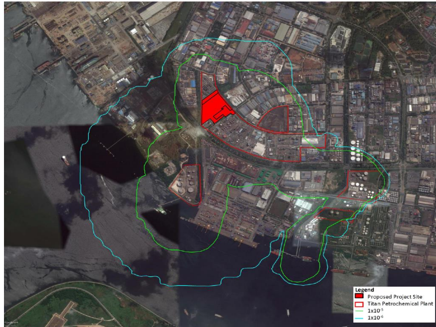
Figure 5-15 Example of Individual Risk Contours using PHAST
