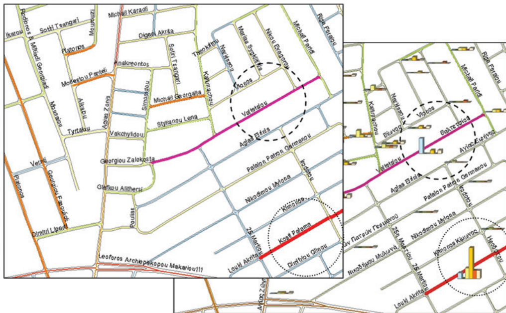
Figure 4.6 Colour-coded GIS mapping of risk-of-failure (Source: Christodoulou et al. , 2007).
