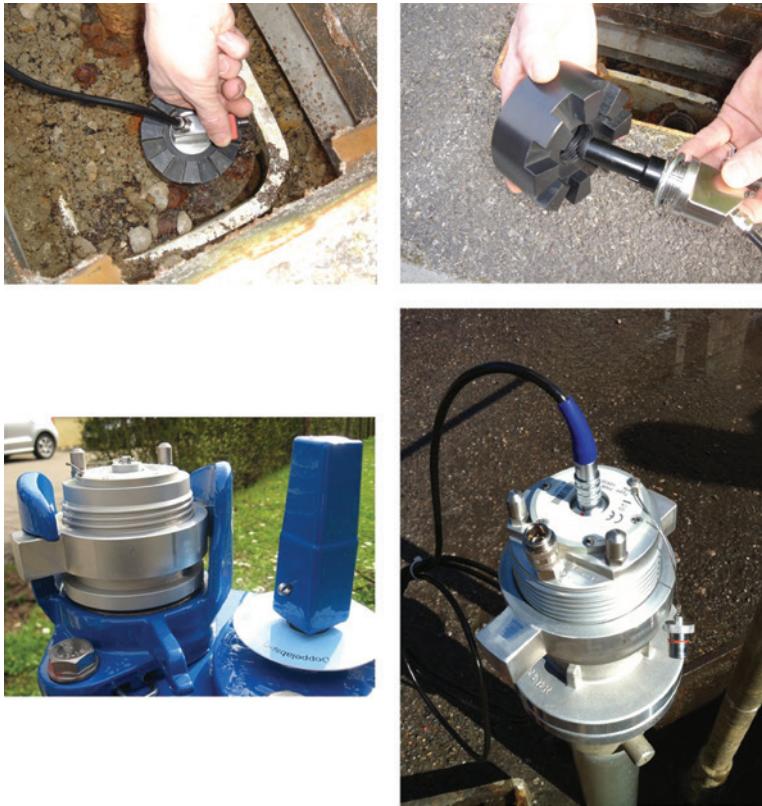
Figure 2.4 Example of hydrophone (source: primayer (top) and seba KMT (bottom)).
