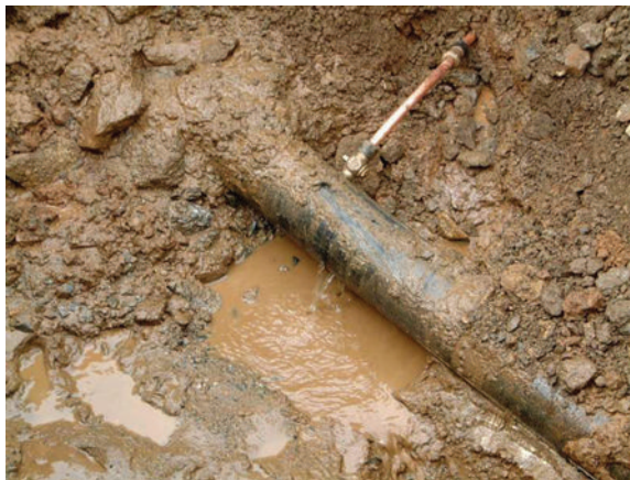
Figure 3.3 Underground leak running at low pressure ( Source: Ken Brothers ).
