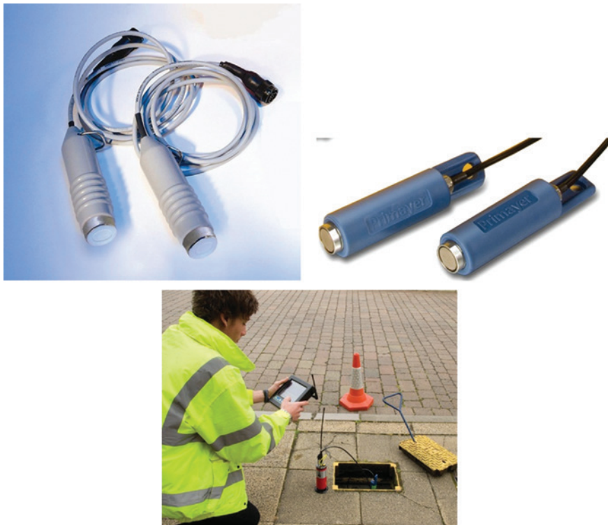
Figure 2.3 Example of accelerometer (Source: Halma Water Management (left) and primayer (right and bottom)).
