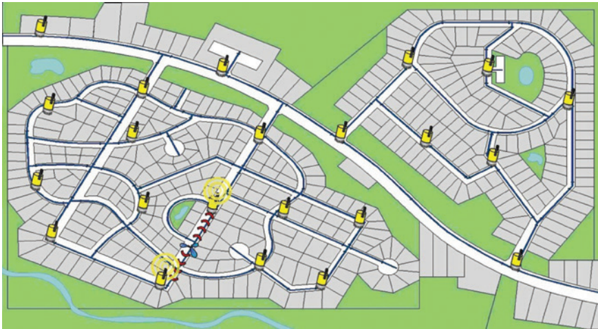
Figure 2.9 Noise logger schematic (Source: Halma Water Management).
