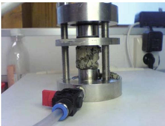
Fig. 2.11 Typical failure with oblique shear planes formed at uniaxial compression of dense clastic clay with a high content of clay particles <2\mu\text{m}
