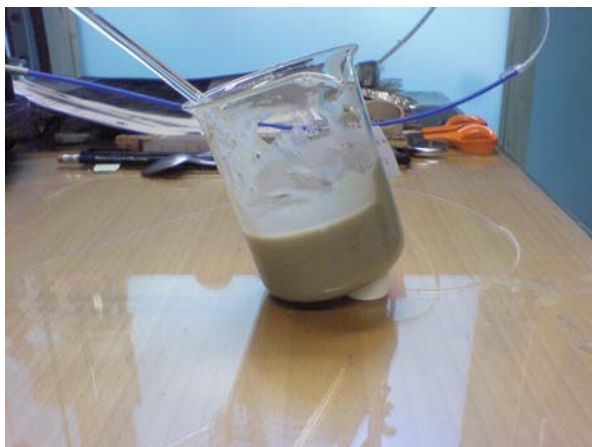
Fig. 3.26 Clay mud of MX-80 bentonite with the density 1100 \text{ kg/m}^3 prepared by mixing clay powder with distilled water and left to rest for 2 minutes. The shear strength is sufficient to avoid “slope failure” of the clay gel
