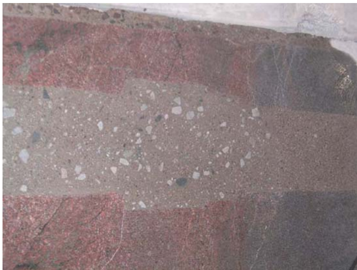
Fig. 4.66 Mechanical seals at the upper ends of deep boreholes. Upper: Copper plug of expander type for placement and prestressing in reamed boreholes. Lower: Sectioned concrete plug (porphyry-like) cast in reamed boreholes with 200 mm diameter [12]
