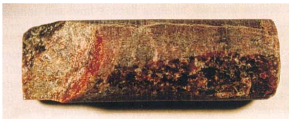
Fig. 2.4 Example of fracturing in the boring-disturbed wall of a 5 m diameter TBM tunnel in granite. The core has a diameter of 10 mm and a length of about 16 mm. The coring was made perpendicularly to the wall surface. Notice the axial fissures and the ones parallel to the oblique fracture surface [4]
