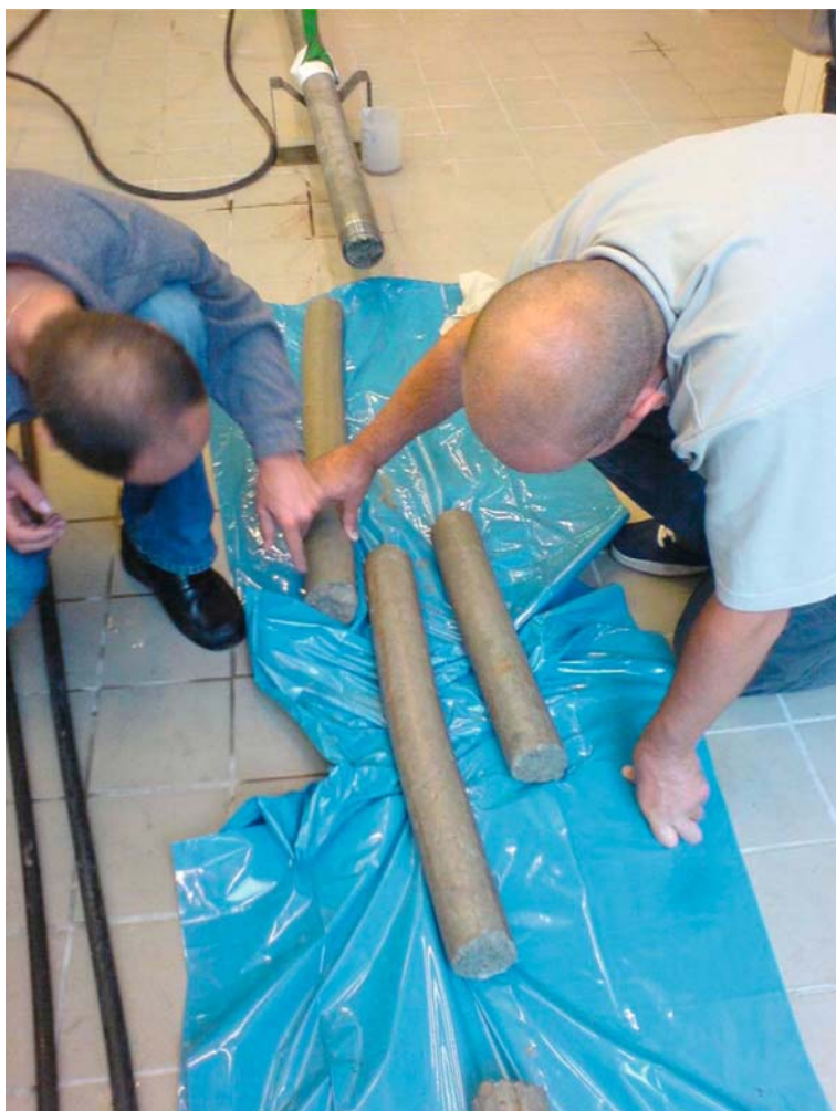
Fig. 4.72 Appearance of the “Pellet” plug extruded from the tube used in the laboratory for simulating a borehole in the “piping” test. Notice the coherence of the plug which broke by mechanical strain at the expulsion
